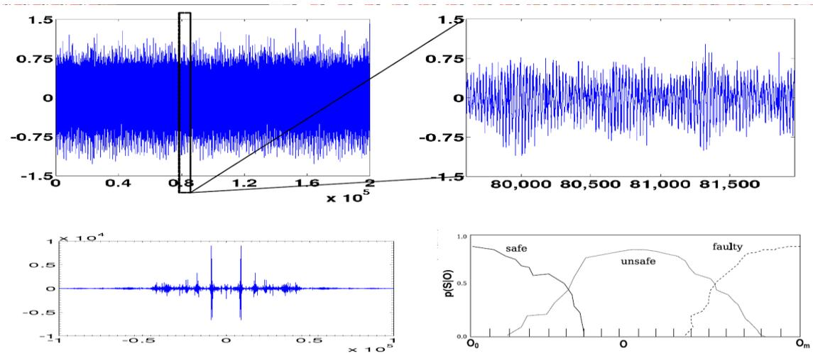
Figure 3. Real-time data from the transmission system of a helicopter's rotor. The top component of the figure presents the original data stream (left) and an enlarged time slice (right). The lower left figure is the result of the Fourier transform of the time slice data (transformed) into the frequency domain. The lower right figure represents the hidden states of the helicopter rotor system.
