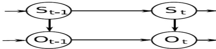
Figure 4. The data of Figure 3 is processed using an auto-regressive hidden Markov model. States  $\mathbf{O}_t$  represent the observable values at time  $t$ . The  $\mathbf{S}_t$  states represent the hidden "health" states of the rotor system, {safe, unsafe, faulty} at time  $t$ .
