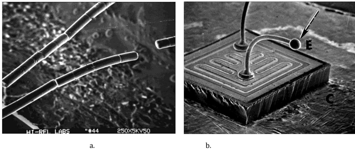
Figure 1. Two examples of discrete component semiconductors, each exhibiting the “open” or “connection broken” failure.
